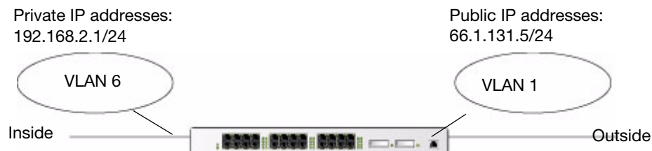
Figure 8 Example: Source NAT using Switch IP Address
